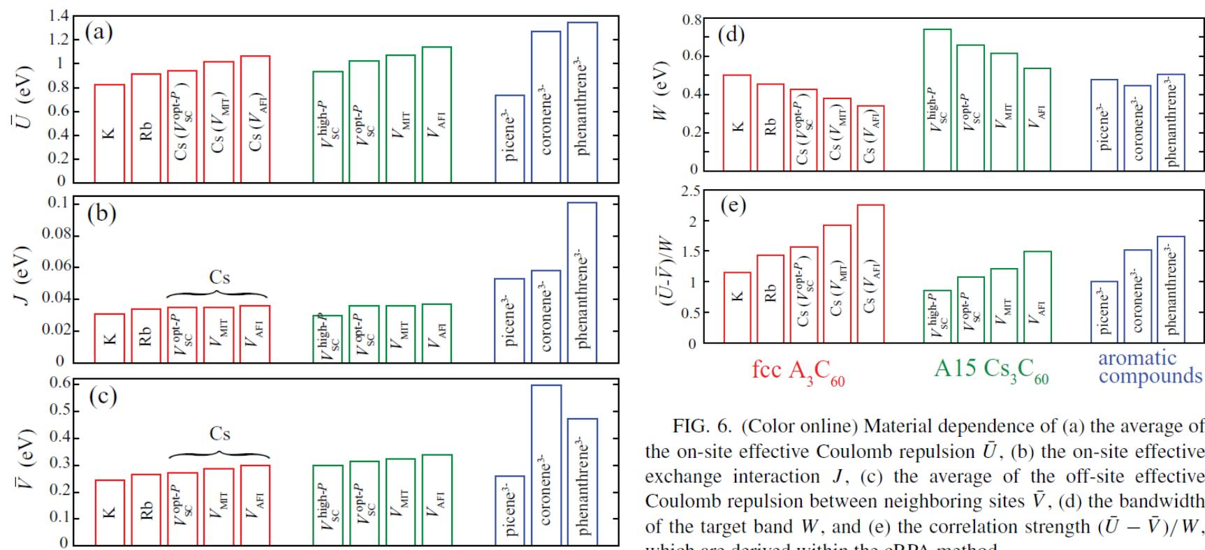
FIG. 6. (Color online) Material dependence of (a) the average of the on-site effective Coulomb repulsion  $\bar{U}$ , (b) the on-site effective exchange interaction  $J$ , (c) the average of the off-site effective Coulomb repulsion between neighboring sites  $\bar{V}$ , (d) the bandwidth of the target band  $W$ , and (e) the correlation strength  $(\bar{U} - \bar{V})/W$ , which are derived within the crRPA method.
